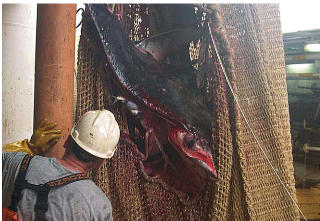
Fig. 3. Manta ray entangled in the filter grid after a regular (non-excluder) commercial set; note rope pulling the “zipper” junction that enables access inside the trawl.
